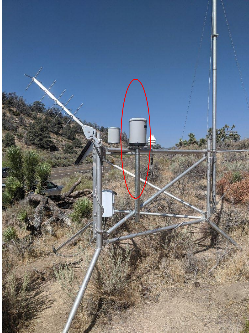
FIGURE 1. TIPPING BUCKET RAIN GAUGE INSTALLATION AT WALKER PASS EAST RAWS
